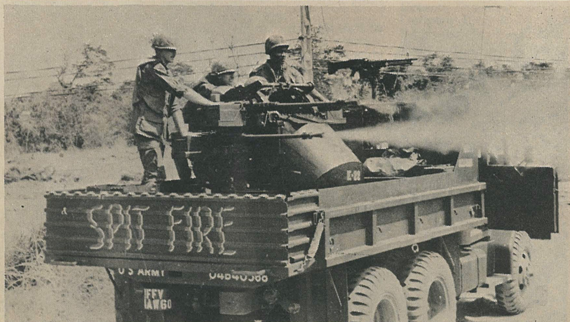
MOBILITY —A rolling arsenal of firepower, soldiers from Echo Company, 41st Artillery (Quad 50s) blaze away from their truck bed called Spit Fire. The four mounted .50 calibre machine guns and the mounted M60 do just that—spit fire and hot lead as they help bolster perimeter defenses and convoys with the mobile concentration of heavy fire.
